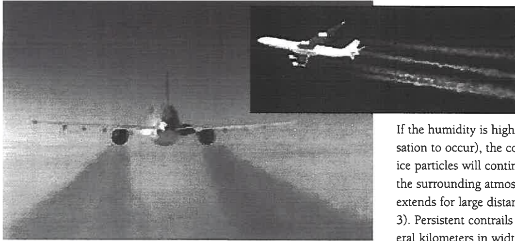
Figure 1. Contrails forming behind the engines of a Lufthansa Airbus A310-330 cruising at an altitude of 35,100 ft (10.7 km) as seen from research aircraft. (Photo: German Aerospace Center (Deutsches Zentrum für Luft- und Raumfahrt (DLR)), Oberpfaffenhofen, Germany.) Inset: Contrails forming behind the engines of a large commercial aircraft. Typically, contrails become visible within roughly a wingspan distance behind the aircraft. (Photo: Masako Imai, Cloud Castle/Photo Sky Japan.)
